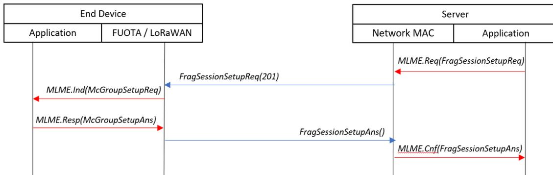
Figure 5: Fragmented data block transport session initialisation for firmware transmission
